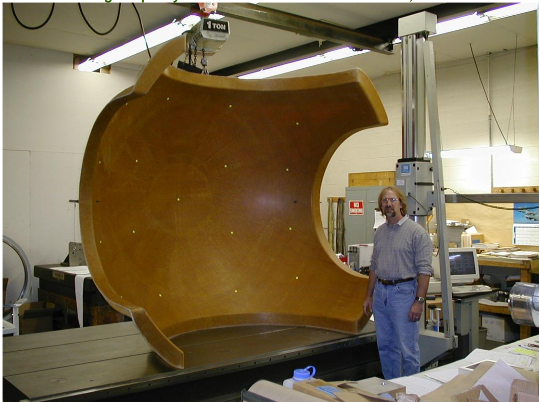
Large Capacity CMM 132" X 48" Y 78" Z max wt. 10,000 Lb.
