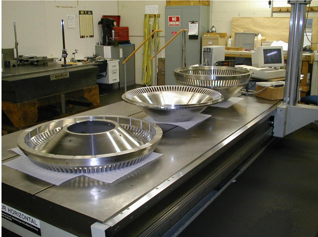
Large Capacity CMM 132" X 48" Y 78" Z max wt. 10,000 Lb.
