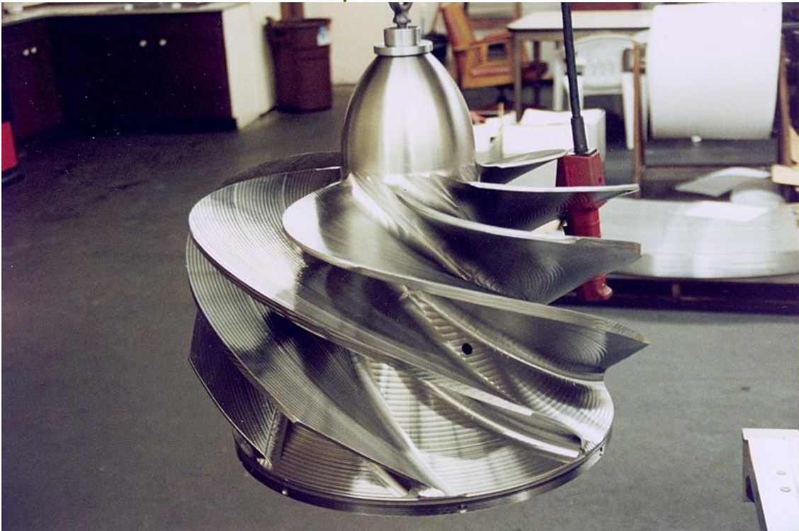
26 Inch Diameter Titanium Impeller Machined From 3D CAD Database
